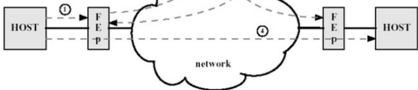
Figure 5.10 Automatic Key Distribution for Connection-Oriented Protocol
